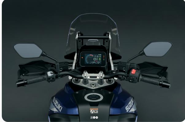
The V-Strom 1050 uses a new custom 5-inch colour TFT display that features clearly legible information displays. The high-quality display keeps you fully aware of all the bike's systems and settings and supplies vital real time operating status information. The tachometer does double duty as a programmable rpm indicator light that blinks when the engine reaches a pre-set speed, and another new function displays large pop-up alerts and warnings. Manual or automatic switching settings for the day
